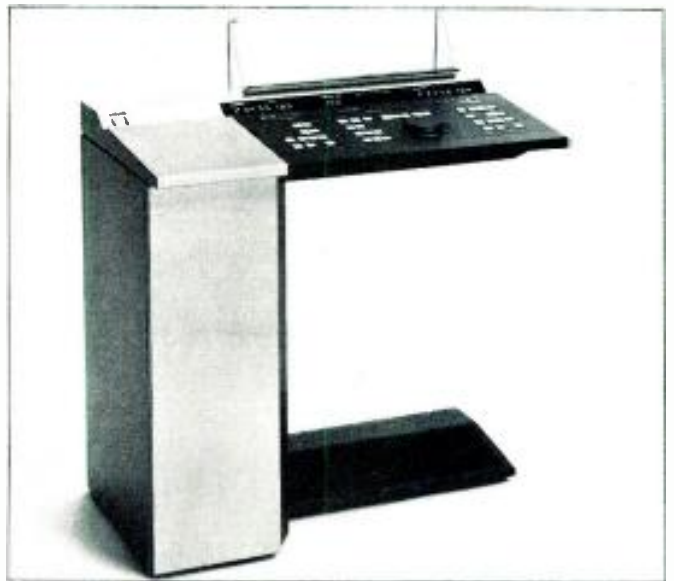
Editing unit developed by Sony for "pseudo-video" recordings of PCM digital audio on video cassettes. Unit allows precise punch-ins, assembly edits, etc., with matched signal amplitudes
