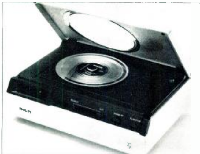
The Philips "Compact Disc," which uses a four-inch disc recorded and played back by a laser beam, is one of several digital phono systems which are ready to bring the digital revolution to the home—only lack of standardization holds them back
